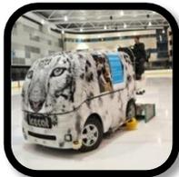
As the Ice Cat lays down a layer of fresh water to freeze and smooth the ice, it scrapes the top layer of ice from the rink and transports it to be recycled
